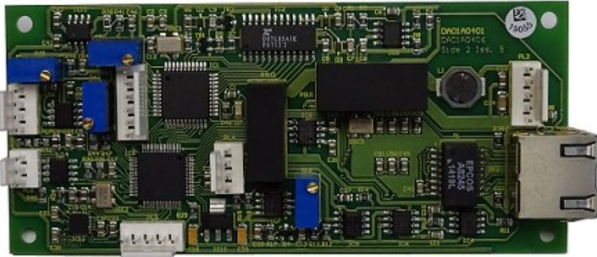
*Figure 1: Ethernet Board Top Side*
