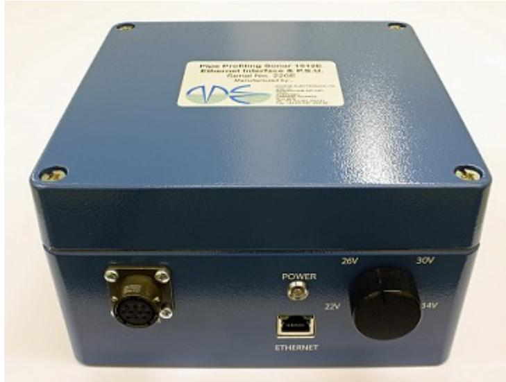
Figure 4: Ethernet Surface Box
