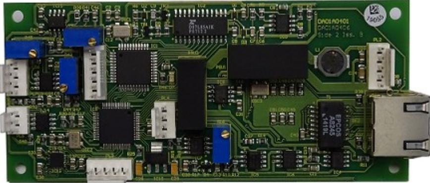
Figure 12: Ethernet Board Top Side
